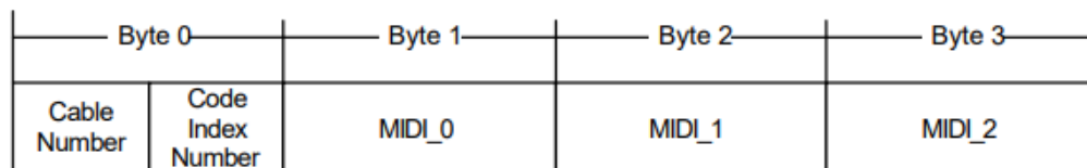
Figure 11: 32-bit USB-MIDI Event Packet Description (USB, 1999).
